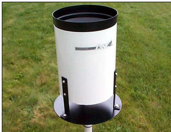
260-2501-A Rain Gauge with 260-950 Mounting Plate
